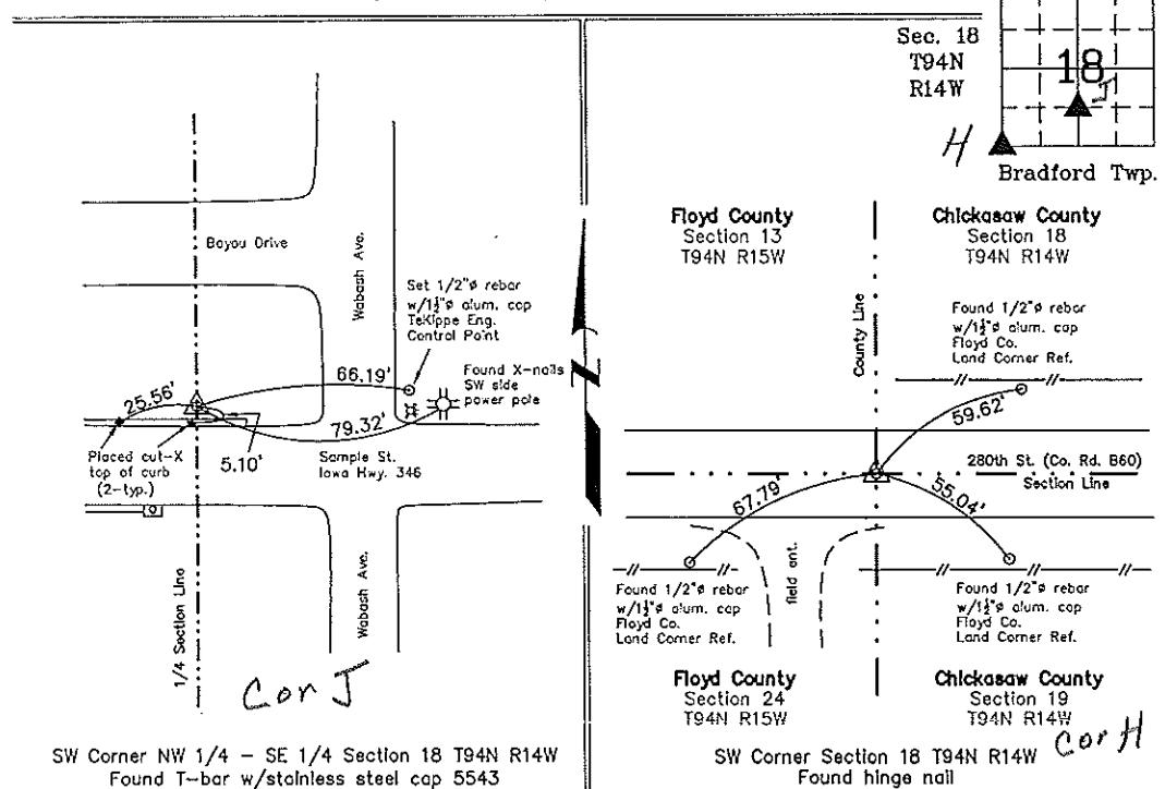
SW Corner NW 1/4 - SE 1/4 Section 18 T94N R14W
