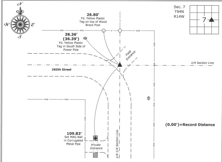
Southeast Corner SW 1/4 - NE 1/4 of Section 7-94-14 Found 1/2"Ø Rebar w/2"Ø Aluminum Cap PLS 16961
