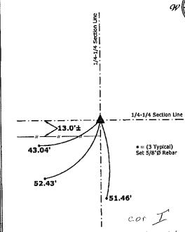
1.) Northeast Corner SW 1/4-SW 1/4 Section 1-95-14 Set 5/8\*Ø rebar w/2\*Ø aluminum cap PLS 15525 21.23'
