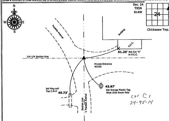
Southeast Corner NE 1/4-NE 1/4 Section 24-95-14 Set 5/8\*Ø rebar w/2\*Ø aluminum cap PLS 15525
