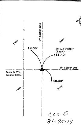
1.) Center of Section 31-95-14 Set 5/8"Ø rebar w/2"Ø aluminum cap PLS 15525
