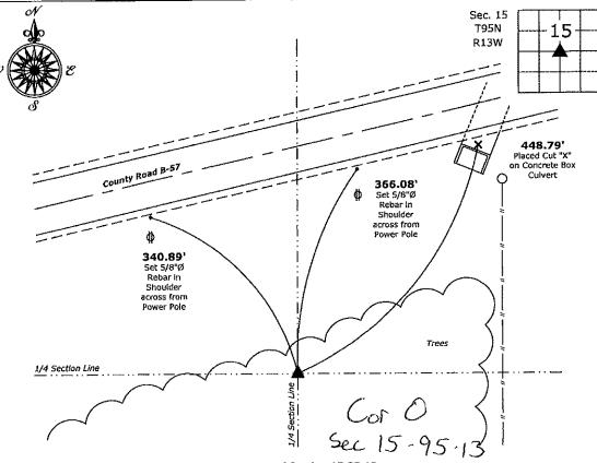
Center of Section 15-95-13 Set 5/8"Ø rebar w/2"Ø aluminum cap PLS 19211
