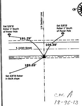
1.) South 1/4 Section 18-95-13 Set 5/8"Ø rebar w/2"Ø aluminum cap PLS 19211
