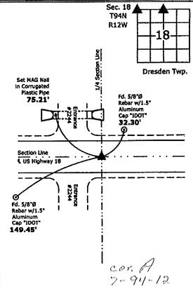
2.) North 1/4 Corner Section 18-94-12 Fd. Survey Mark Nail w/Stainless Steel Washer \*IDOT\*
