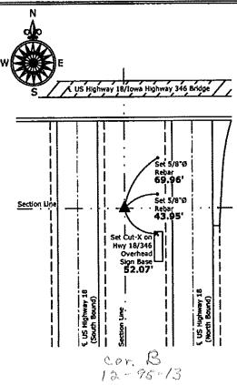
1.) Northwest Corner Section 18-94-12 Fd. 5/8°Ø Rebar w/1.5° Aluminum Cap "IDOT"
