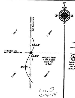
1.) Center Section 16-96-14 Set 5/8"Ø rebar w/2"Ø aluminum cap PLS 19211
