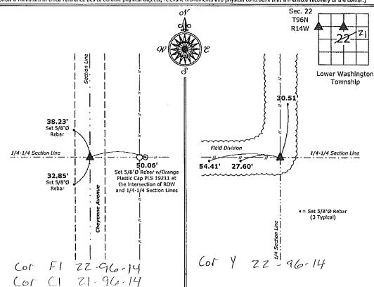
1.) Northwest Corner SW 1/4-NW 1/4 Section 22-96-14 Set 5/8"Ø rebar w/2"Ø aluminum cap PLS 19211
