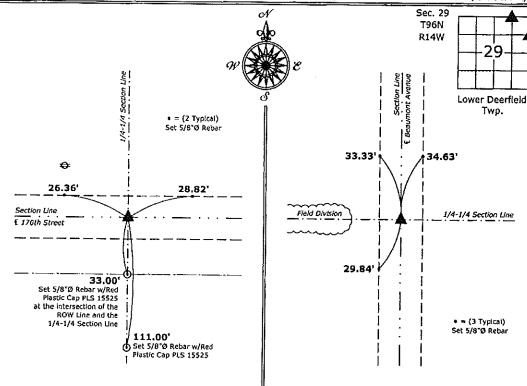
1.) Northeast Corner NW 1/4-NE 1/4 Section 29-96-14 Set 5/8°Ø rebar w/2°Ø aluminum cap PLS 15525
