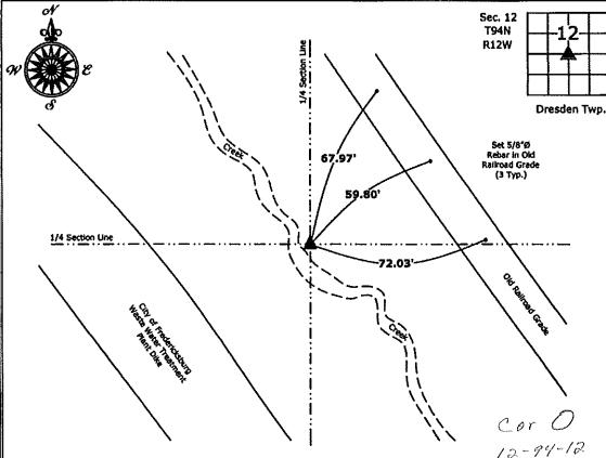
Center of Section 12-94-12 Set 5/8"Ø rebar w/2"Ø aluminum cap PLS 19211
