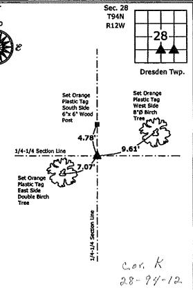
1.) Northeast Corner SE 1/4-5W 1/4 Section 28-94-12 Set 5/8\*Ø rebar w/2\*Ø aluminum cap PLS 15525 2.) Northeast Corner SW 1/4-SE 1/4 Section 28-94-12 Set 5/8\*Ø rebar w/2\*Ø aluminum cap PLS 15525
