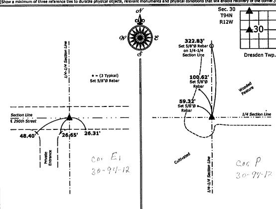
1.) Northeast Corner NW 1/4-NW 1/4 Section 30-94-12 Set 5/8"Ø rebar w/2"Ø aluminum cap PLS 15525
