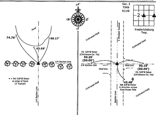
1.) Center of Section 2-94-11 Set 5/8\*Ø rebar w/2\*Ø aluminum cap PLS 19211
