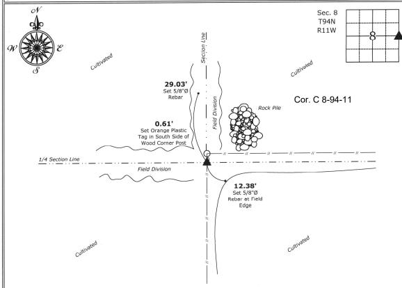
East 1/4 Corner of Section 8-94-11 Set 5/8"Ø rebar w/2"Ø aluminum cap PLS 19211
