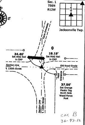
2.) Northeast Corner Section 1-96-12 Set 5/8\*Ø rebar w/2\*Ø aluminum cap PLS 15525
