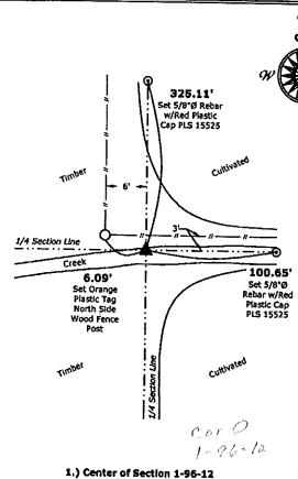
1.) Center of Section 1-96-12 Set 5/8"Ø rebar w/2"Ø aluminum cap PLS 15525
