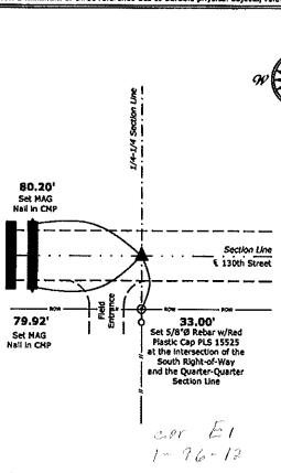
Jacksonville Twp. 80.20 Set MAG Nail in CHE Section Line £ 130th Street 79.92 33.00 Set MAG Set 5/8°Ø Rebar w/Red Nall In CMP Plastic Cap PLS 15525 at the intersection of the South Right-of-Way and the Quarter-Quarter Section Une 36-97-12
