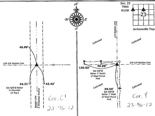
1.) Northwest Corner SW 1/4-NW 1/4 Section 23-96-12 Set 5/8"Ø rebar w/2"Ø aluminum cap PLS 19211
