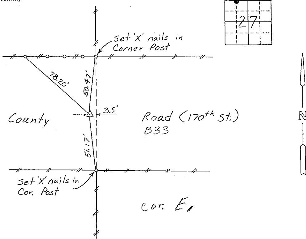
NE CORNER, NW 1/4 - NW 1/4, SECTION 27-T96N-R12W
