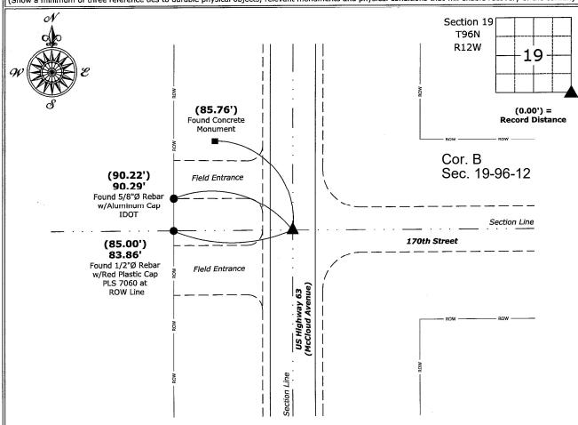
**Southeast Corner of Section 19-96-12**Found Survey Mark Nail w/Stainless Steel Washer IDOT
