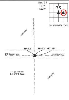
1.) Center of Section 35-97-12 Set 5/8"Ø rebar w/2"Ø aluminum cap PLS 15525 2.) Southeast Corner SW 1/4-NE 1/4 Section 35-97-12 Set 5/8"Ø rebar w/2"Ø aluminum cap PLS 15525
