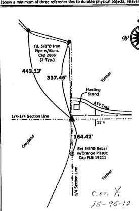
1.) Northwest Corner SE 1/4-NW 1/4 Section 15-95-12 Set 5/8\*Ø rebar w/2\*Ø aluminum cap PLS 19211
