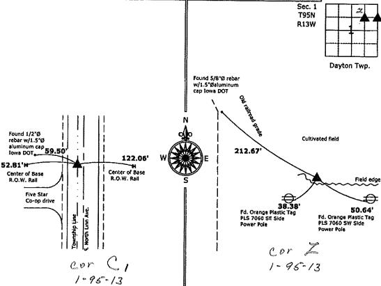
1.) NE Corner SE 1/4-NE 1/4 of Section 1-95-13 Found Cut-X 2.) NE Corner SW 1/4-NE 1/4 of Section 1-95-13 Found 1/2\*Ø rebar
