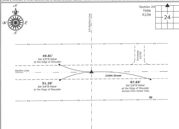
North 1/4 Corner of Section 24-95-12 Set 5/8"Ø Rebar w/2"Ø Aluminum Cap PLS 19211
