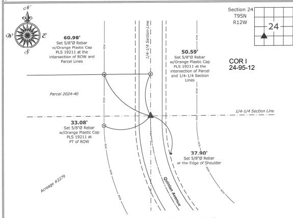
Northeast Corner of the SW 1/4 - SW 1/4 of Section 24-95-12 Set 5/8"Ø Rebar w/2"Ø Aluminum Cap PLS 19211
