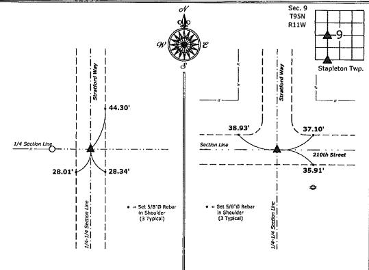
1.) Northeast Corner NW 1/4-SW 1/4 Section 9-95-11 Set 5/8°Ø rebar w/2°Ø aluminum cap PLS 19211 2.) Southeast Corner SW 1/4-SW 1/4 Section 9-95-11 Set 5/8\*Ø rebar w/2\*Ø aluminum cap PLS 19211
