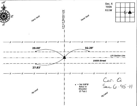
Southwest Corner SE 1/4 - NE 1/4 of Section 6-95-11 Set 5/8"Ø rebar w/2"Ø aluminum cap PLS 19211
