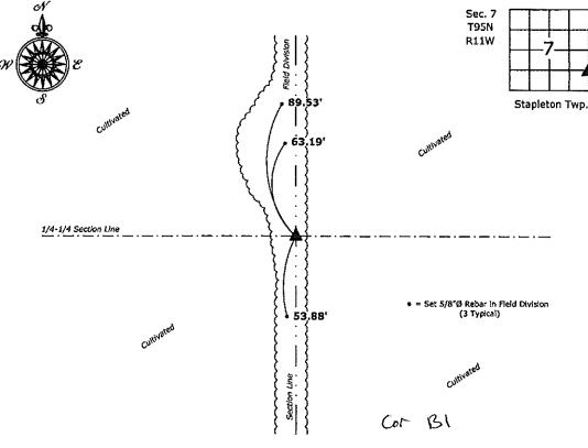
Southeast Corner NE 1/4-SE 1/4 Section 7-95-11 Set 5/8"Ø rebar w/2"Ø aluminum cap PLS 19211
