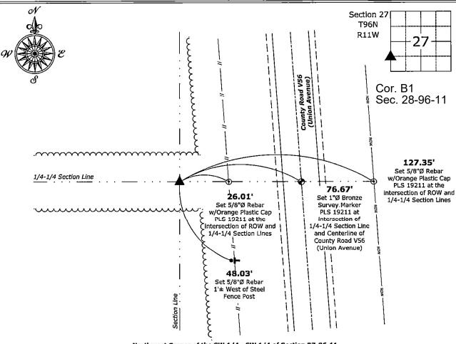
Northwest Corner of the SW 1/4 - SW 1/4 of Section 27-96-11 Set 5/8"Ø Rebar w/2"Ø Aluminum Cap PLS 19211
