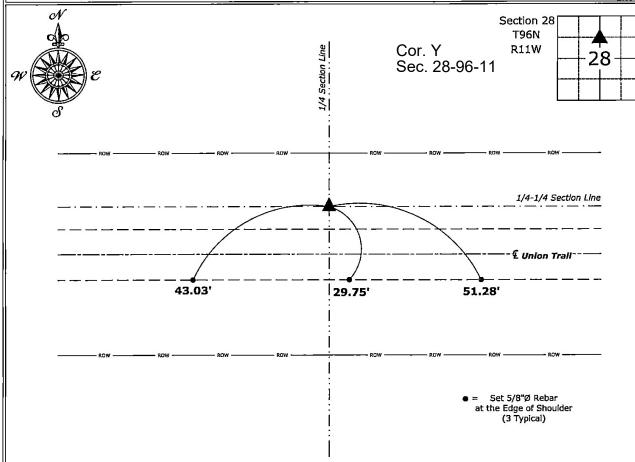
Southwest Corner of the NW 1/4 - NE 1/4 of Section 28-96-11 Set 5/8"Ø Rebar w/2"Ø Aluminum Cap PLS 19211
