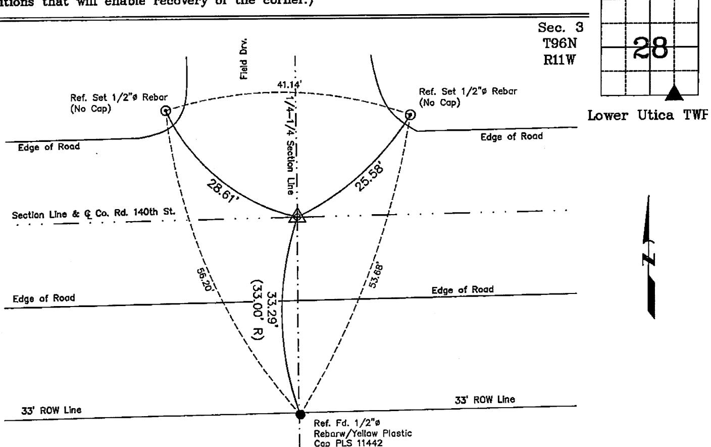
SW Corner of the SE 1/4 — SE 1/4 of Section 3-T96N-R11W
