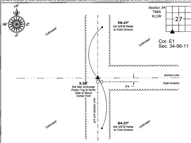
Southeast Corner of the SW 1/4 - SW 1/4 of Section 34-96-11 Set 5/8"Ø Rebar w/2"Ø Aluminum Cap PLS 19211
