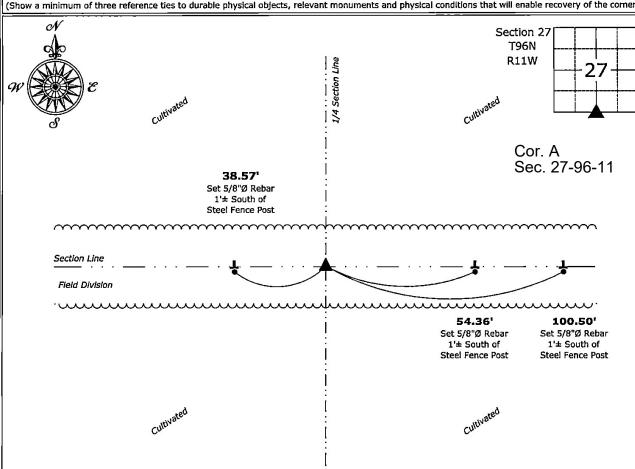
South 1/4 Corner of Section 27-96-11 Set 5/8"Ø Rebar w/2"Ø Aluminum Cap PLS 19211
