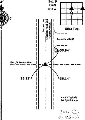
1.) Southwest Corner NW 1/4-NE 1/4 Section 9-96-11 Set 5/8\*Ø rebar w/2\*Ø aluminum cap PLS 15525 2.) Southeast Corner NE 1/4-NE 1/4 Section 9-96-11 Set Survey Mark Nail w/Stainless Steel Washer PLS 15525
