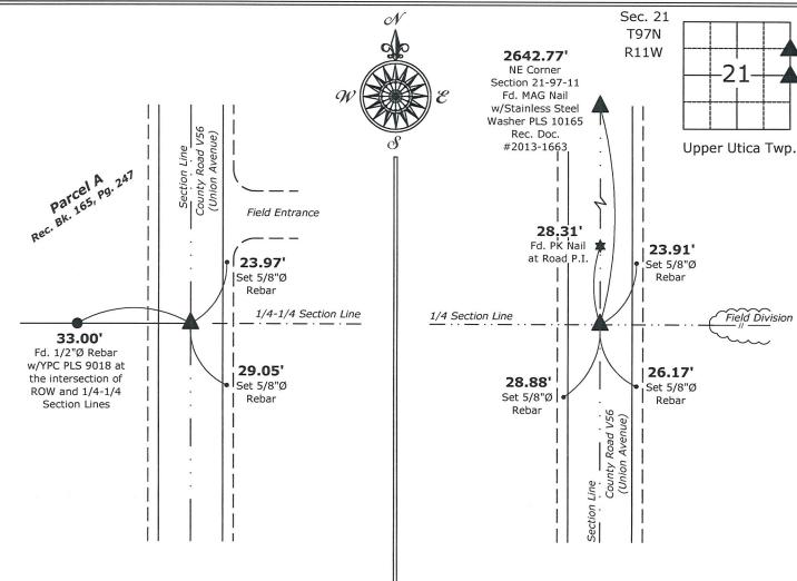
1.) Southeast Corner NE 1/4-NE 1/4 Section 21-97-11 Set Survey Mark Nail w/Stainless Steel Washer PLS 19211 2.) East Quarter Corner Section 21-97-11 Set Survey Mark Nail w/Stainless Steel Washer PLS 19211
