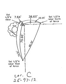
W 1/4 Corner Section 30 T97N R11W Found 1/2"ø rebar w/yellow plastic cap 11442
