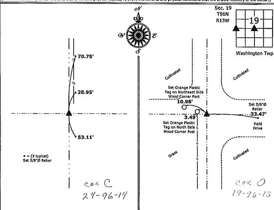
1.) West 1/4 Corner 19-96-13 Set 5/8"Ø rebar w/2"Ø aluminum cap PLS 15525 2.) Center Section 19-96-13 Set 5/8\*Ø rebar w/2\*Ø aluminum cap PLS 15525
