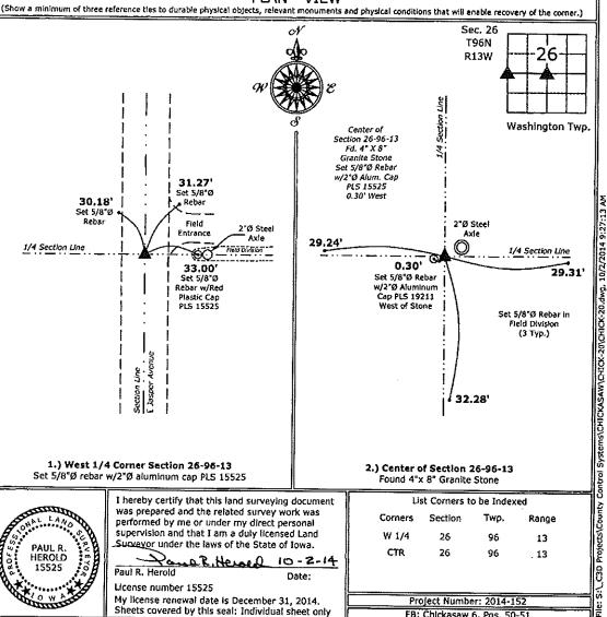
1.) West 1/4 Corner Section 26-96-13 Set 5/8"Ø rebar w/2"Ø aluminum cap PLS 15525
