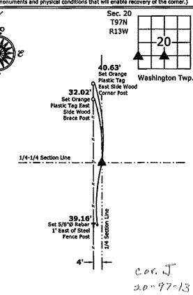
1.) Northwest Corner SW 1/4-SW 1/4 Section 20-97-13 Set 5/8\*Ø rebar w/2\*Ø aluminum cap PLS 15525 2.) Northeast Corner SE 1/4-SW 1/4 Section 20-97-13 Set 5/8\*Ø rebar w/2\*Ø aluminum cap PLS 15525
