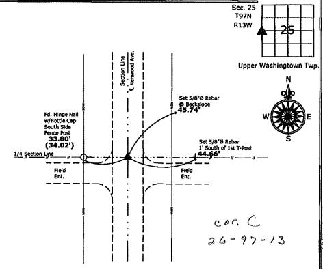
West 1/4 Corner Section 25-97-13 Found 3/4" square bar (bent), Replaced with 5/8"Ø rebar w/2"Ø aluminum cap PLS 19211 at straight portion location
