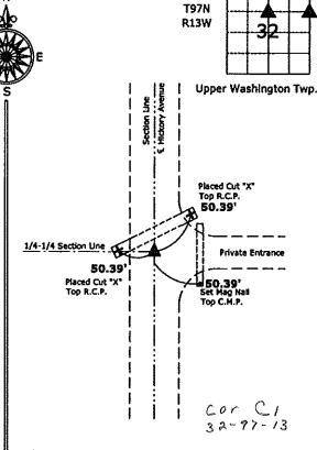
2.) Northeast Corner SE 1/4-NE 1/4 Section 32-97-13 Set 5/8"Ø rebar w/2"Ø aluminium cap PLS 15525
