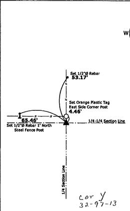
1.) Northwest Corner SW 1/4-NE 1/4 Section 32-97-13 Set 5/8\*Ø rebar w/2\*Ø aluminium cap PLS 15525
